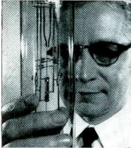
Dr. Volney C. Wilson inspects one of his experimental thermionic converters.
