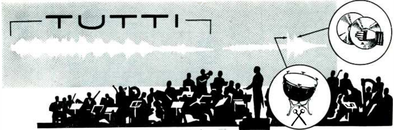
Fig. 35. Oscillogram of pickup output showing the full orchestra at the left, which is then followed by drums and cymbals.
