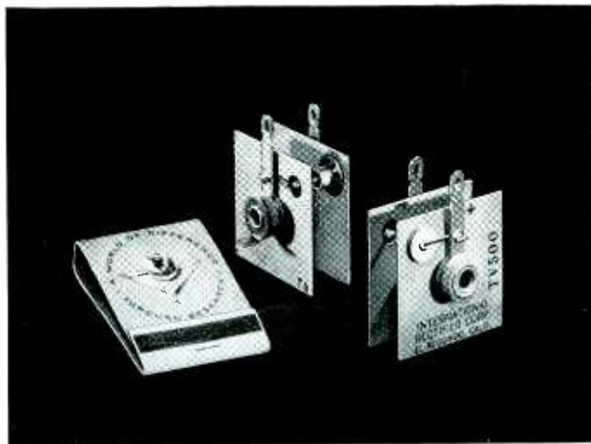
Fig. 3. The International Rectifier's silicon "Unistac."
